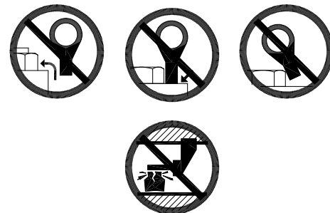
FIGURE 4-4B IMPROPER REACTION POINTS/POSITIONS FOR THE RSL REACTION ARM WITH THE SQUARE DRIVE WRENCH HEAD
